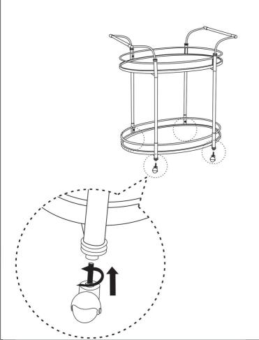
Step 2: Parts B screw to Part A
